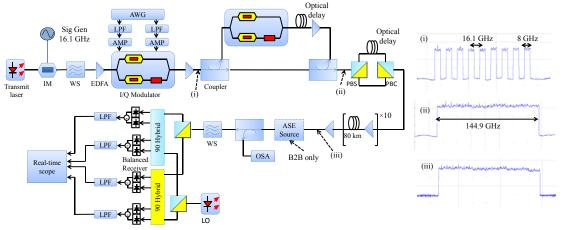
Fig. 2. Experimental setup for 1.15 Tb/s Nyquist PDM-16QAM system.
