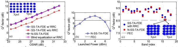
Fig. 3. Measured Q<sup>2</sup>-factor of: (a) 9<sup>th</sup> band versus OSNR in B2B transmission with different equalization schemes, (b) 13<sup>th</sup> band versus launched power after 800-km transmission with N-SS-TA-FDE, and (c) all bands after 800-km using SS-TA-FDE with RRC or N-SS-TA-FDE.
